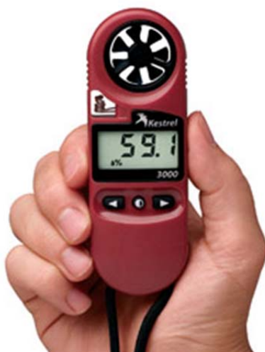
Figure 1 – TasNetworks issued (portable) Kestrel 3000 used for assessing weather conditions while onsite
