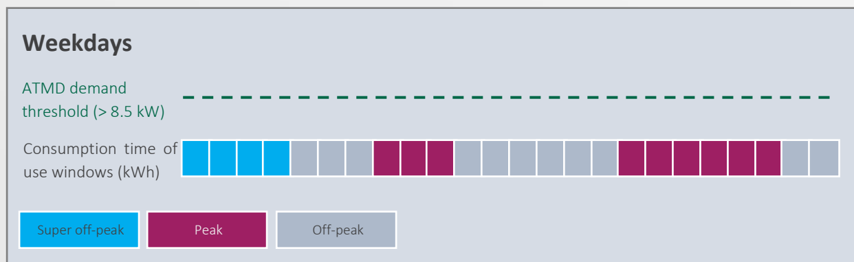
Figure 1 Proposed structure of the residential time of use DER network tariff (TAS97)
