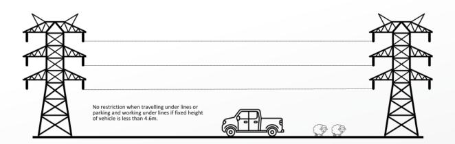
Vehicles with a fixed height of less than 4.6m (utes, tractors, trucks, harvesters)
