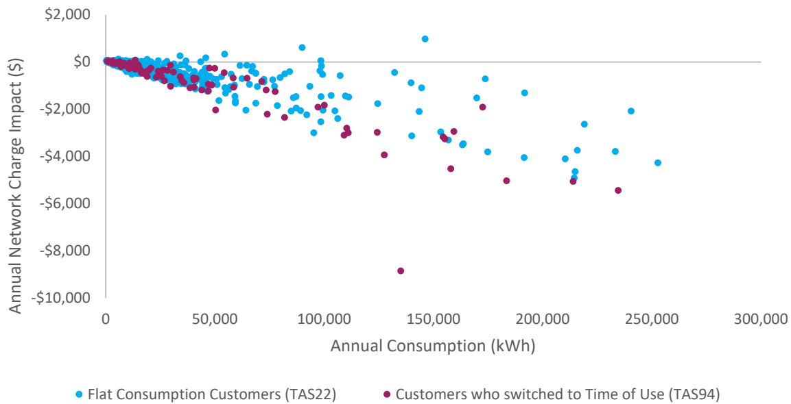
Figure 20 – Annual network charge for Time of Use Consumption (TAS94) vs Flat Rate Consumption Tariff (TAS22)
