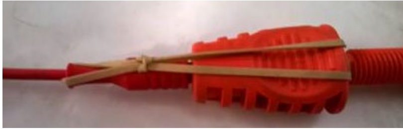
Rubber bands or tape can be used to keep the test probe connected.
