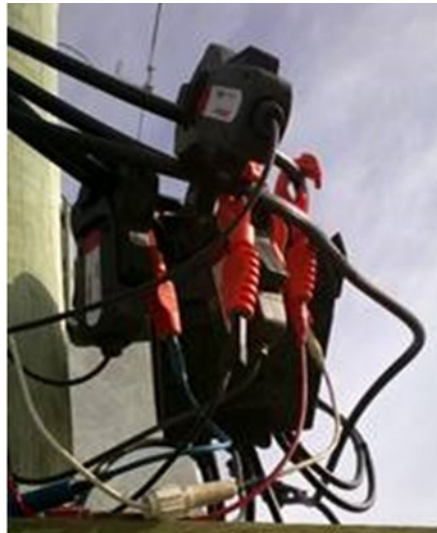
Rubber bands or tape can be used to keep the test probe connected.
