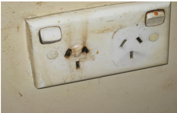
Burnt out power point socket
