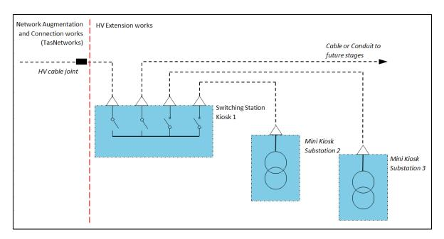
Figure 5: HV switching station with 2 remote mini kiosks.
