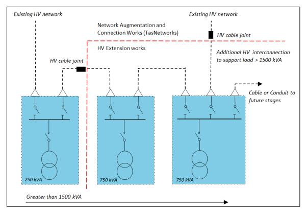
Figure 6: HV Interconnector using a 3way HV switchboard arrangement.
