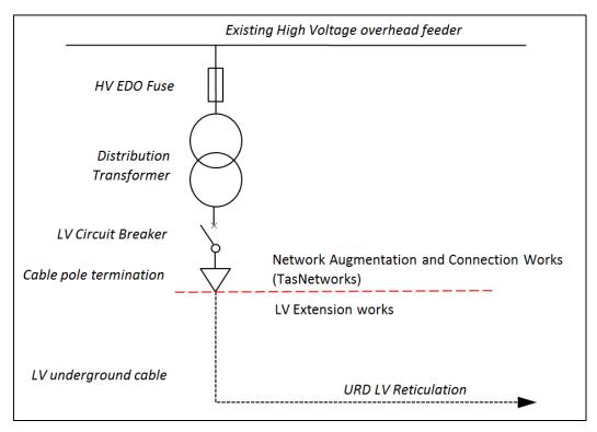
Figure 1: LV connection from pole mounted transformer.
