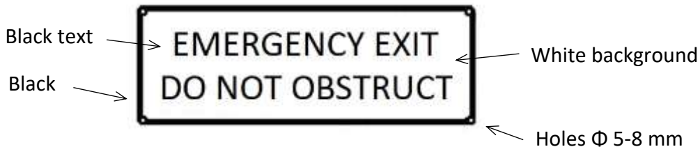
Figure 4 : Emergency exit, Do not obstruct sign.
